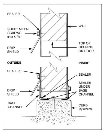
Many rubber-based sealer compounds are not intended for use in areas of strong sunlight since ultraviolet light rays and solar heat gain can cause early deterioration of these compounds. The recommended joint and trim sealer for outdoor applications is McGill AirSeal's UL-Classified UNI-WEATHER<sup>™</sup> duct sealer, which provides long-term ultraviolet, heat, and ozone resistance.
