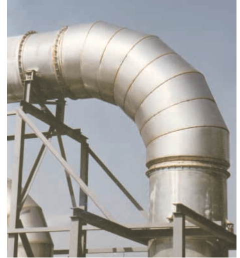
The 64-inch diameter ACOUSTI-k27 elbow is constructed of aluminized heat-resistant steel and lined with thermal insulation wool.
